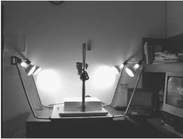
FIG. 1. Components of the digital image system with uniform illumination for in vitro plantlet sample image production.
